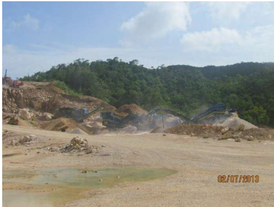
Plate 11: Crushing and Screening System in Series
