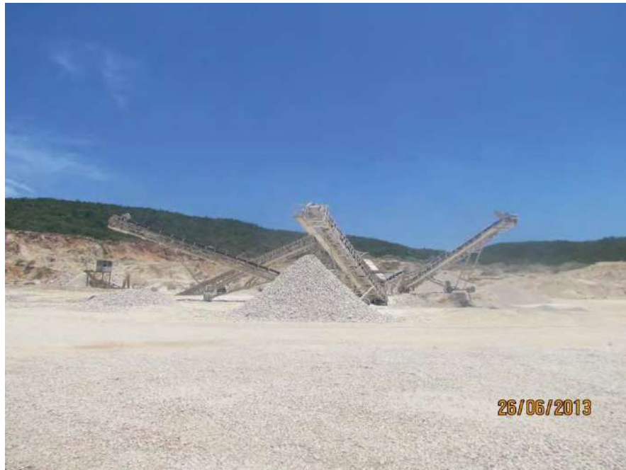
Plate 9: Conventional Crushing and Screening Systems
