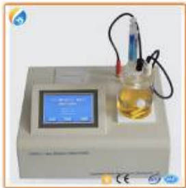
Transformer Oil Water Content Tester/Karl Fischer Titrator Oil Moisture Analyzer
